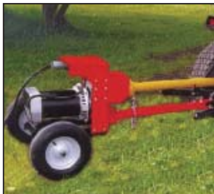
Left: This is one example of a Power Take Off generator which is attached to a tractor. Above: Portable generators require the use of extension cords to run from appliances to the generator.
